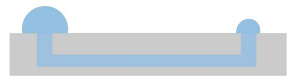
Surface energy will drive the liquid to the end of the tube. The interfacial energy of the air-solid interface exceeds that of the liquid-solid interface. To minimize its total energy the system therefore rearranges such that the air-solid interfacial area is minimized.
